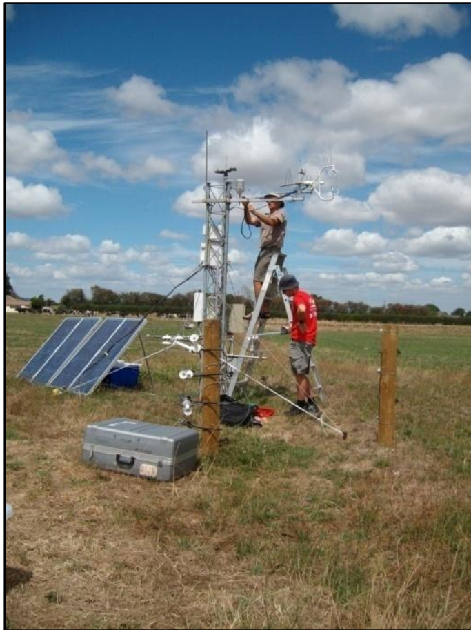
Figure 3.5 Installation of eddy covariance instrumentation.
